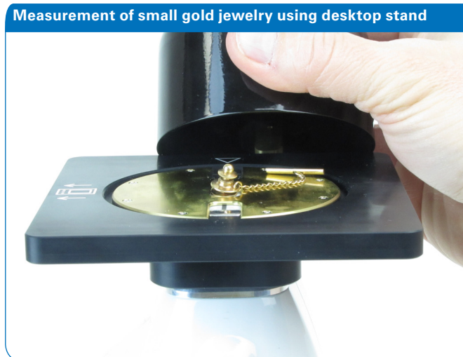
Use of the optional desktop-top stand with the S1 TURBO enables precise sample positioning
